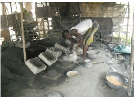
Making cooking pots from aluminium cans melted down
