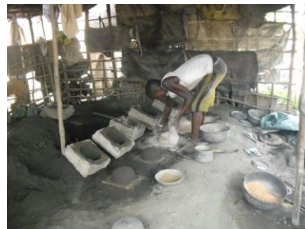
Making cooking pots out of aluminium cans melted down
